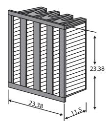
Industrial Grade Plastic Frame with Double Wall Construction
